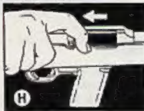
Pull charging handle all the way back. Let it snap forward freely.
